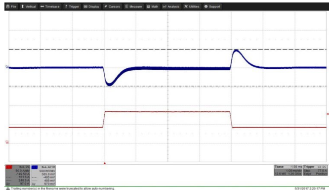
Fig. 30: Output voltage response to load current step change 50% - 100%- 50% (42A–84A–42A) with di/dt = 1A/\mu s at V_{in} = 14V . Top trace (C4): Output voltage (500 mV/div.). Bottom trace (C3): Load current (50A/div.). Time: 1ms/div.
